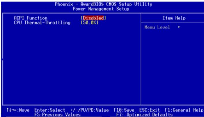
*Figure 4.6: Power Management Setup Screen*
