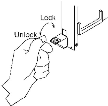
**Figure 2.5: Installing/Removing the MIC-3316 into/from the Chassis**
