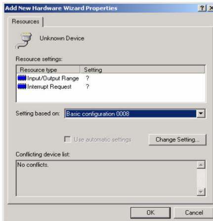
**Step 11** Set Resources Input/Output Range 03F8-03FF / Interrupt Request 04 and “OK”.
