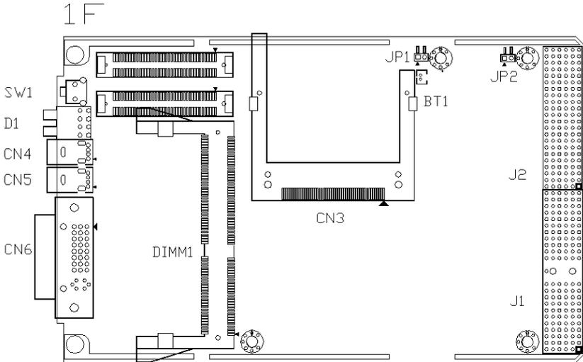
**Figure 2.1: MIC-3316 Connector Locations (1F)**
