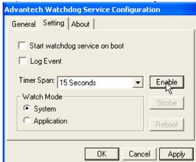
Step 6: Check the Start watchdog service on boot to enable the Watchdog timer to start automatically after the system boots every time.
