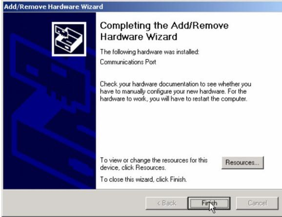
**Step 14** Repeat <Step2>~<Step11> to add another COM In Step 10 to set Resources Input/Output Range 02F8-02FF / Interrupt Request 04
