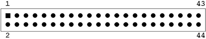
For direct installation of 2.5" IDE HDD (2F-CN17)
