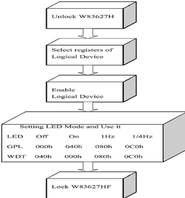
**Figure B.1: Flow Chart for LED Programming**
