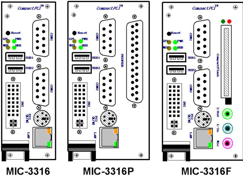
Figure 2.4: MIC-3316 Front Panel Connector and Indicator Locations
