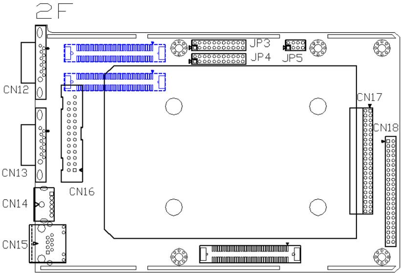
**Figure 2.2: MIC-3316 Connector Locations (2F)**
